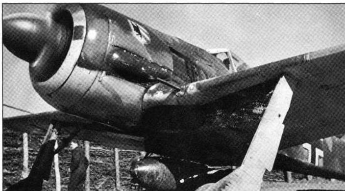
A bomb-carrying Fw 190 seen in the spring of 1943. The weapon mounted to the centreline ventral stores rack is an SB 500 kg High Explosive (HE) bomb. This type of weapon was the favoured ordnance for the Gruppe on the Russian Front, although a single SB 1000 kg bomb could also be carried, as well as smaller 250 and multiple 50 kg devices
