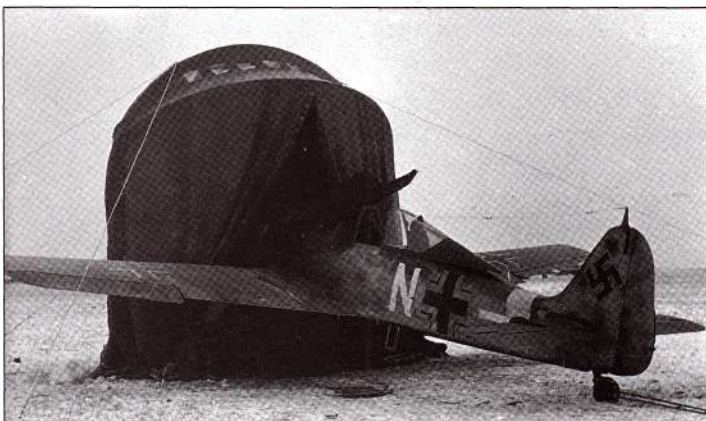
Above and right What the well-dressed Fw 190F wore in the depths of winter. Heating trollies and tents were available only for the lucky few! The latter were often reserved for aircraft undergoing in-the-field maintenance, as conditions often proved too bitter in the depths of winter for 'black men' to work outdoors for any period of time. Note that 'White N' has had a toned down cross applied to its fuselage, although its overall effect is spoiled somewhat by the full-colour Staffel markings
