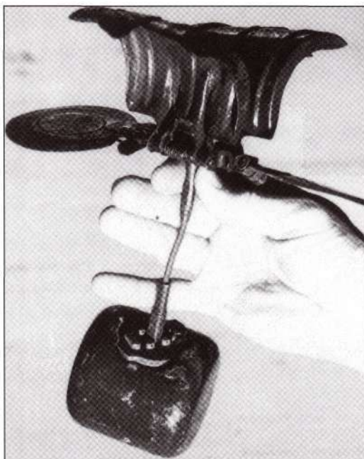
The SD-2 Splitterbombe in its fully-armed state. After release, the outer casing's two clamshell halves sprang open to form a kind of parachute to retard the bomb's fall. They in turn freed a pair of circular discs which acted as a wind vane as they rotated about, and moved up, the short steel cable. This action fused the bomb's 7.5-oz (212-gr) charge of TNT
